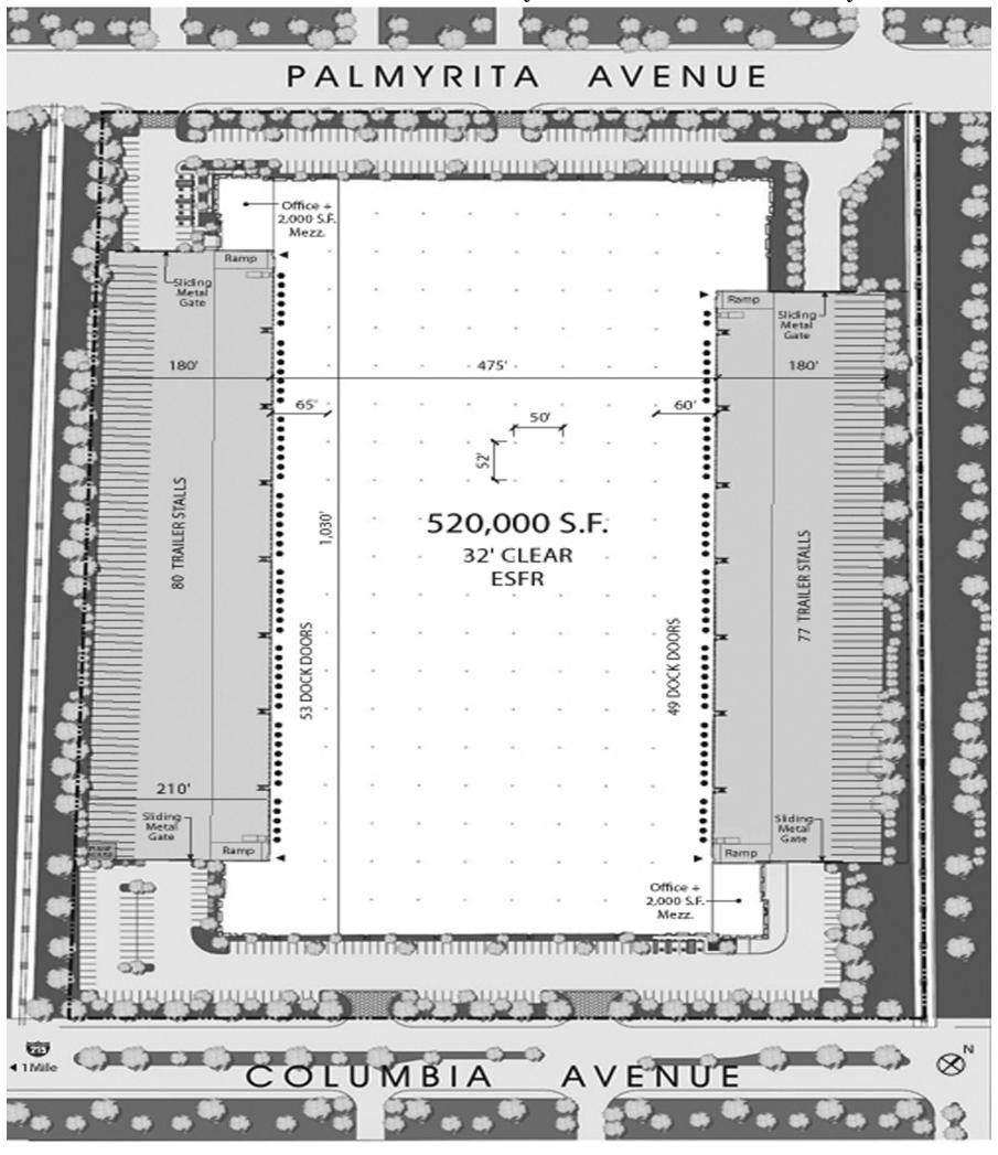
25 acres are currently being graded for this giant 520,000 Sq. Ft. cross dock warehouse that stretches from Palmyrita Ave. all the way to Columbia Avenue. The plan above shows 53 dock doors on the west side and 49 on the east side for 102 dock doors. It also shows 80 trailer stalls on the west side and 77 trailer stalls on the east side for a total of 157 trailer stall parking spaces. The verticle left hand margin of the above plan is where the Perris Valley Line Railroad track is located-
