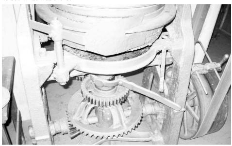
Here is a view of the gears that are engaged when the wind blows against the blades of the fan. In the Vogel Paint windmill the fan and gears were used in the paint making process back in the 1920's.
