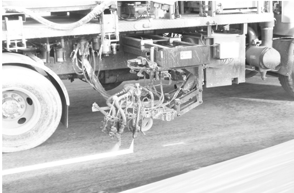
Here is a close-up of the truck! Crushed glass helps us see the lines at night.
