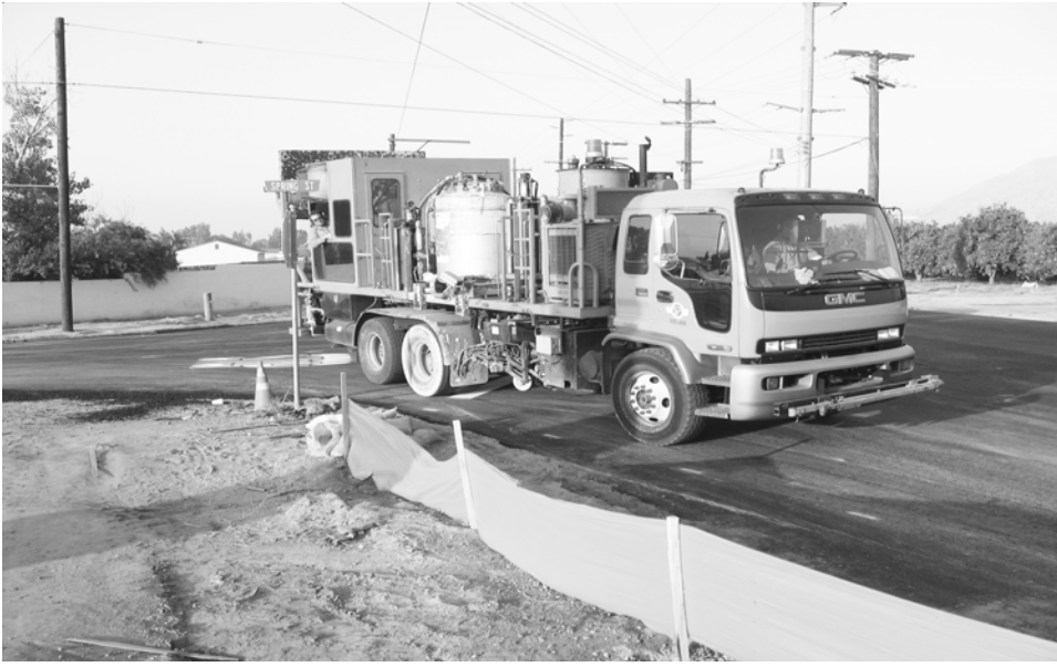
This truck is used to paint the lines in the road. The paint operator is shown at the rear of the truck in his compartment. Communication between the driver and the painter is essential to put the lines where they belong.
