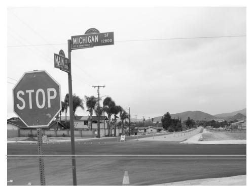
The intersection at Main St. and Michigan Ave. will get a new traffic signal. The width of Main St. is 46 feet with 30 feet on the north side of Main St. for 2 westbound lanes and a width of 14 feet for 1 eastbound lane on the south side of the street. Some locations along Main St. are even wider.
