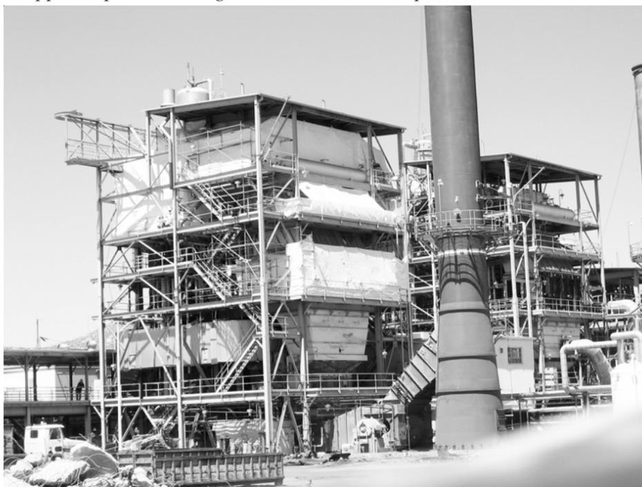
The white plastic prevents asbestos from contaminating the air.
