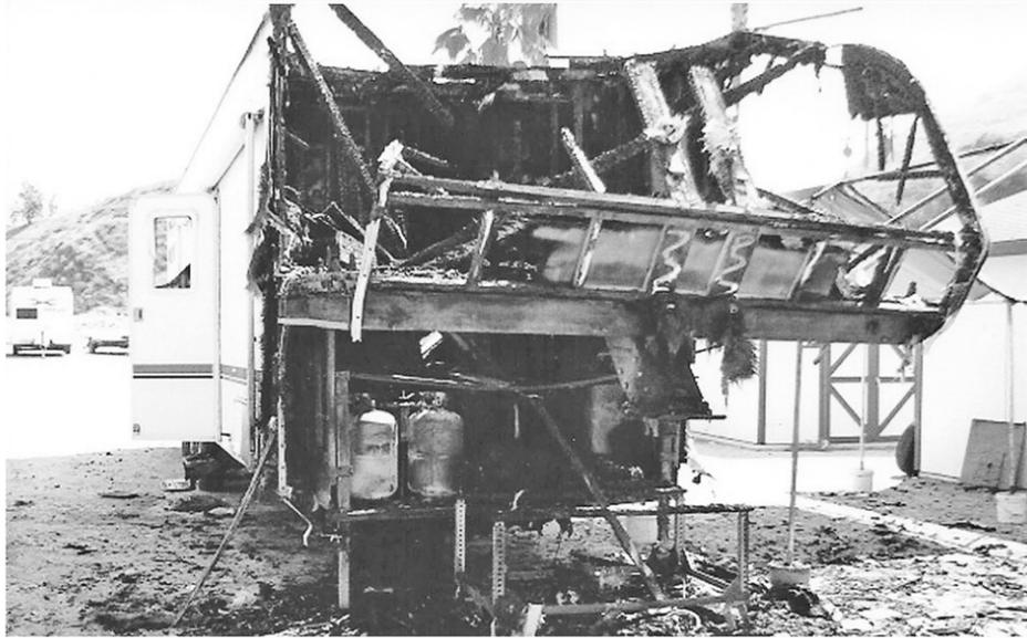
Faulty wiring was blamed for causing the fire that destroyed this unoccupied 5th wheel in Reche Canyon but luckily the propane tanks did not explode.
